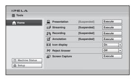
2 Use the ♠, ♣, ♠ or ▶ button to select "Setup", then press the ENTER button on the Remote Commander.
