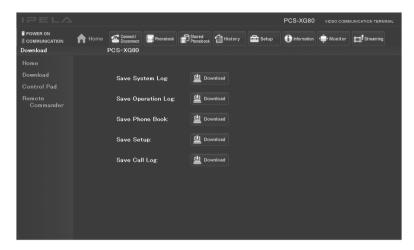
Select the log file you want to display, and click the [Download] button. You can check the log files in a separate window.
