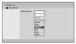
The system begins dialing the remote parties registered in the multipoint connection list. "Dialing" appears on the monitor screen. When the system connects to all the remote points, the message "Session Connected." appears on the screen, and the pictures of the remote parties are displayed on the screen.
