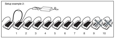
Up to eight microphones are powered by the AC adaptor, counting from the microphone connected to the AC adaptor.
