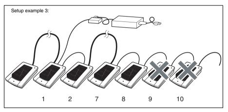
The 8-meter microphone cable is used in the middle of the connections, and counts as four microphones. Up to four microphones are powered by the AC adaptor, counting from the microphone connected to the AC adaptor.
