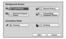
Remote Picture: Selects the picture on the remote site as the background Local Picture: Selects the picture on the local site as the background Received Computer Picture: Selects the computer picture received from the remote site as the background
