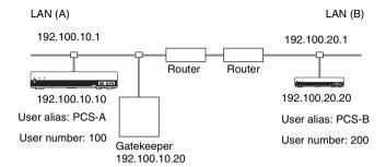
1 Enter a name in "Host Name" under the Basic Setup page in the LAN setup menu, and enter the appropriate values for "IP Address", "Network Mask", and "Gateway Address".
