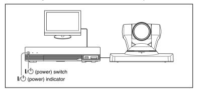
The I/U (power) indicator on the Communication System flashes. The indicator lights in green when the Communication System turns on.
