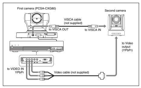
Connect the video output connector on the second camera to the VIDEO IN YPbPr jacks on the front of the Communication System or the S VIDEO IN or RGB IN connector at the rear.
