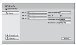
**3** Set up the line interface of the remote parties in the "Dial to:" text boxes. Select the line interface from the drop-down list on the left, and enter the number of a remote party in the text box.
