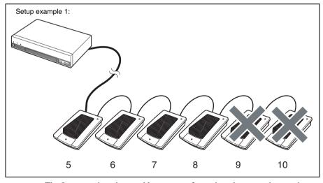
The 8-meter microphone cable counts as four microphones, and power is supplied to only the first four microphones. The same is true if the 8-meter microphone cable is used in the middle of the connections.
