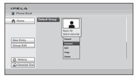
The system begins dialing the selected party. "Dialing" appears on the monitor screen. When the system connects to the system on the remote site, the message "Session Connected." appears on the screen, and the picture on the remote site is displayed.
