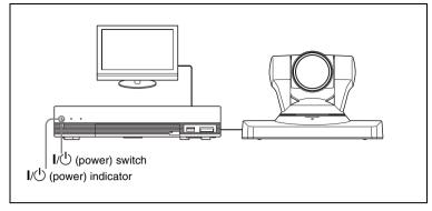
The indicator on the System starts flashing, then lights in green when the power is on.
