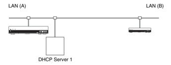
Set "DHCP Mode" to "Auto" under the Basic Setup page in the LAN setup menu.
