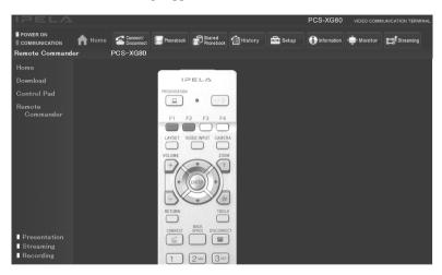
By clicking the various buttons on the Remote Commander image, you can control the system in the same way you can when using a real Remote Commander (PCS-RF1), operating the camera, and dialing phone numbers.
