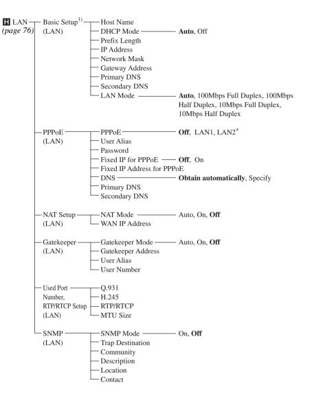
When "Use LAN2" is set to "On" in the Line I/F setup menu, the Basic Setup pages for LAN1 and LAN2 are displayed, and you can set up the items on those pages.
