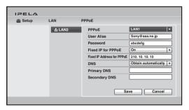
**2** If you have a fixed IP from the provider, set "Fixed IP for PPPoE" to "On", and enter your fixed IP address for PPPoE in "Fixed IP Address for PPPoE" under the PPPoE page in the LAN setup menu.
