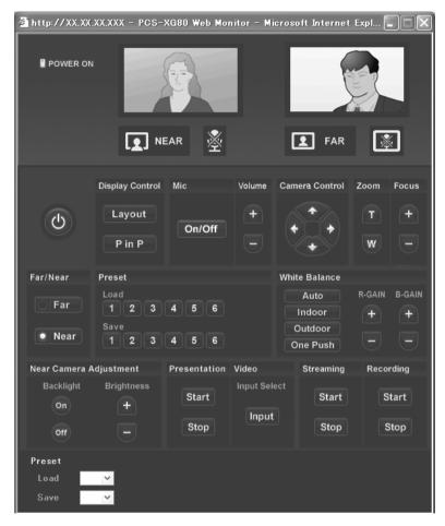
When you click [Monitor] of the tools buttons, the [Monitor] page opens. You can monitor the picture on the Communication System.
