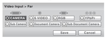
Use the  $\spadesuit$ ,  $\blacktriangledown$  or  $\bigstar$  button on the Remote Commander to select the picture output from the equipment connected to the remote system, then press the ENTER button. The selected picture is input to the local system and is displayed on the monitor screen.
