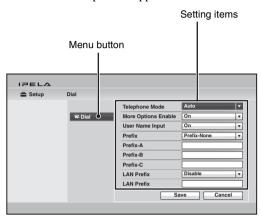
**4** Use the ♠, ♣, ♠ or ▶ button on the Remote Commander to select the setting item, then press the ENTER button.
